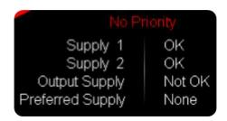
The Home/Status screen shows a mimic diagram and status indication as text. This is the default screen, and a period of inactivity will result in the LCD returning to this location.
