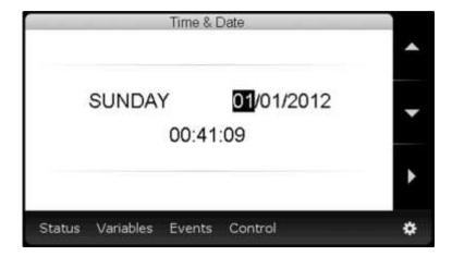
Use the scroll key ▶ to access the parameter then the up & down keys to set the desired parameter values. Parameters are set as soon as they are entered.
