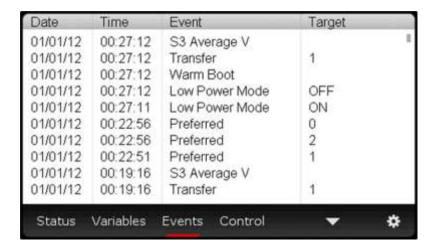
Up to 200 events can be stored. Once the list is full, the oldest events are pushed from the bottom of the list and are replaced by any new events. See the Fault Codes section for more information.
