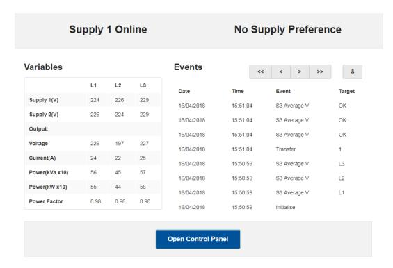
The home page displays the connected supply, supply preference, variables and events list that can be scrolled through using the arrows provided. From the home page, gain access to the Control panel by clicking Open Control Panel and enter following username and password:
